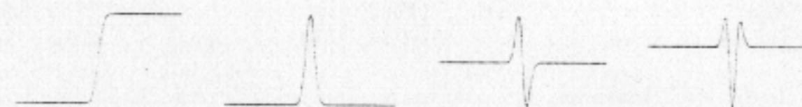
Figure 3.9. (Left to right) A mollified step edge and its 1 st , 2 nd , and 3 rd derivatives.
