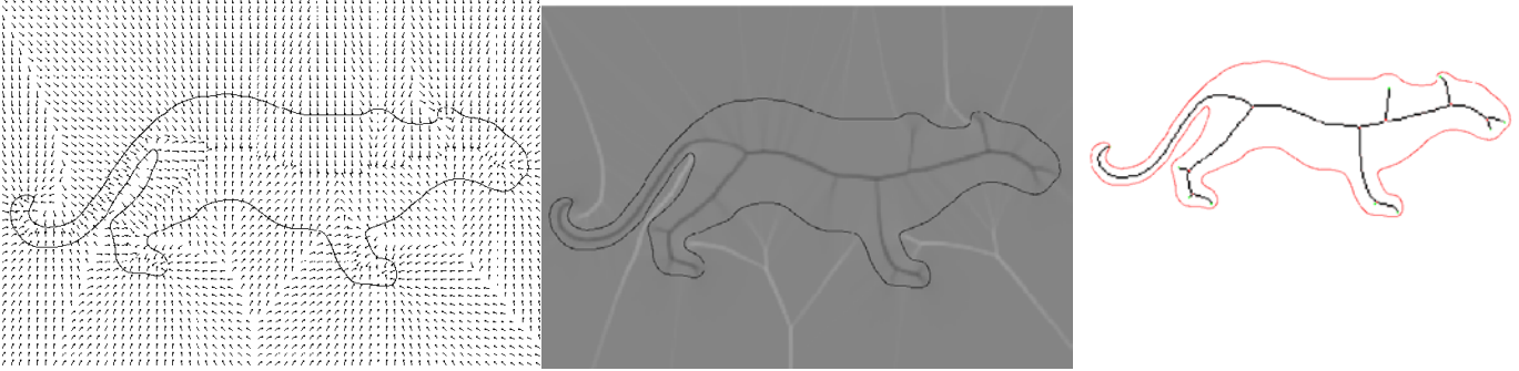
Fig. 6: The gradient vector field of the Euclidean distance function of the boundary of an object (left), the average outward flux (middle) computed over a 3 \times 3 circular neighborhood, and the computed skeleton (right) obtained by homotopy preserving thinning (see Section 5.2).
