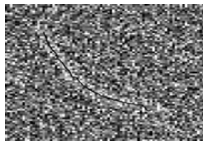
Fig. 3. One slice of a noisy synthetic 3D image of a tube of radius three pixels whose axis lies entirely in the plane displayed. The black curve is the core of the tube.
