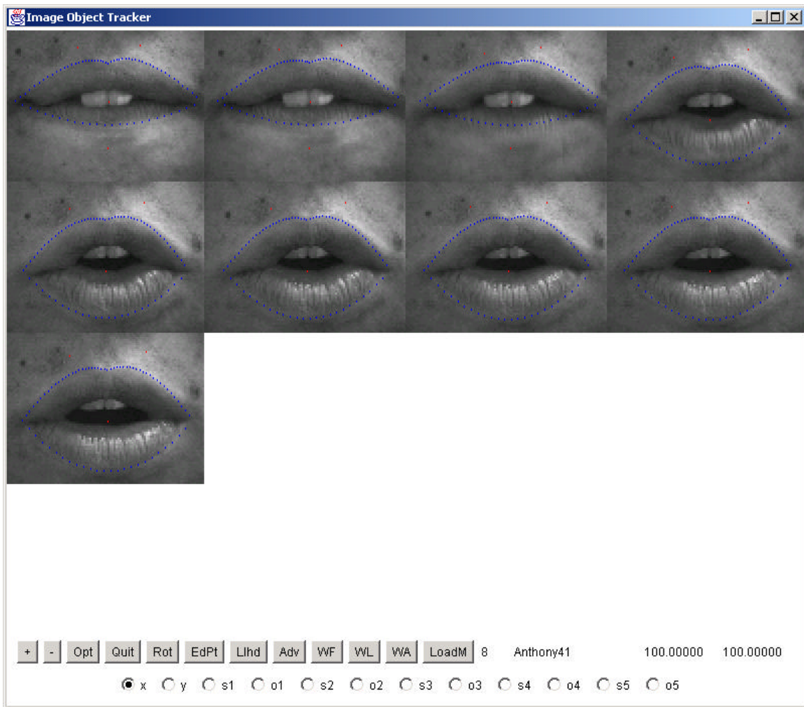
Figure 6.9: Anchor primitive based semi-automatic segmentation of a lip image sequence “four” from talker “Anthony.” The discontinuity observed between frames 3 and 4 above (upper right corner) is typical of the digit “four” for many speakers, because the lower lip accelerates rapidly following release of the plosive.
