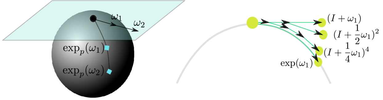
Figure 2.5: Illustration of the exponential map. The exponential map fits a linear tangent plane (actually it is a 3D plane for \mathfrak{so}(3) ) to the identity point of the non-Euclidean space. Vectors in the same direction correspond to a geodesic path in the non-Euclidean space. This allows us to compute derivatives in the tangent space and move the point along a geodesic flow in the non-Euclidean space. This figure is from [74].
