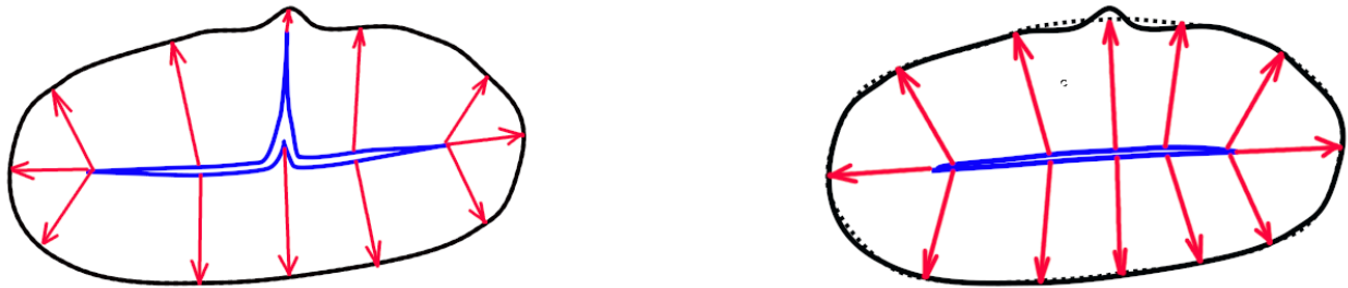
Figure 2.1: Left: a 2D object with non-branching topology except for a boundary bump induced by noise. The noise induces an extra branch on the skeleton (blue). Right: a fitted skeleton to the object that obtains the noise-free object's branching topology. This skeletal model is associated with a slightly modified (dotted) boundary.
